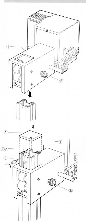
Loosen the carriage lock knob (6) by turning it counter-clockwise. Lift the entire head assembly as shown, matching the column and the opening of the carriage, and put the assembly over the column.
