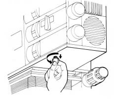
Loosen the screw on the bottom as shown.
