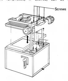
Place the head assembly upsidedown and loosen the four screws with the screwdriver.
